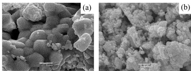
**Fig. 2.** SEM images of (U,Ce)O<sub>2-2</sub> powders prepared from nitric acid solutions under the action of microwave radiation with a power of (a) 800 and (b) 180 W.
