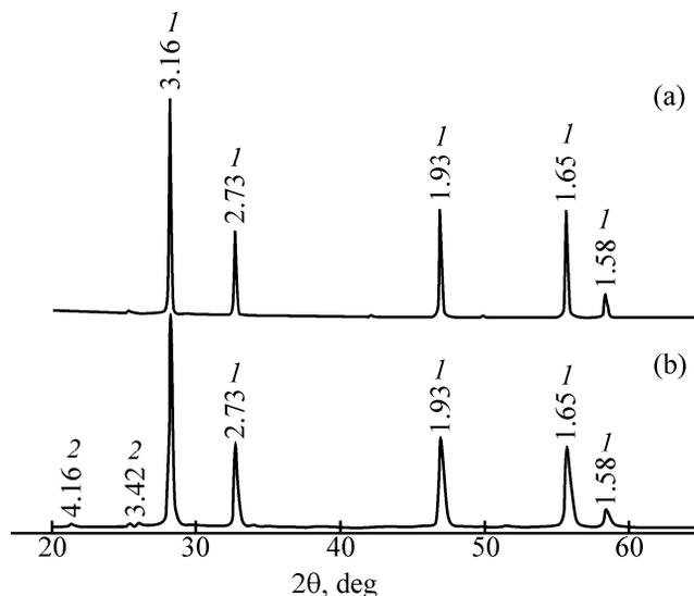
**Fig. 1.** Diffraction patterns of (U,Ce)O<sub>2-2</sub> solid solution powders prepared from nitric acid solutions using microwave radiation with a power of (a) 800 and (b) 180 W. (1) UO<sub>2</sub> (41-1422) and (2) U<sub>3</sub>O<sub>8</sub> (47-1493).
